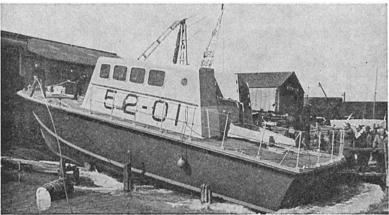
The photograph shows a prototype boat which was launched at Messrs. William Osborne': I buif..fing yard at Little!zampton on 27th March, 1971. This self-righting life-boat has an overall length of 52 feet, a 17 foot beam and a
