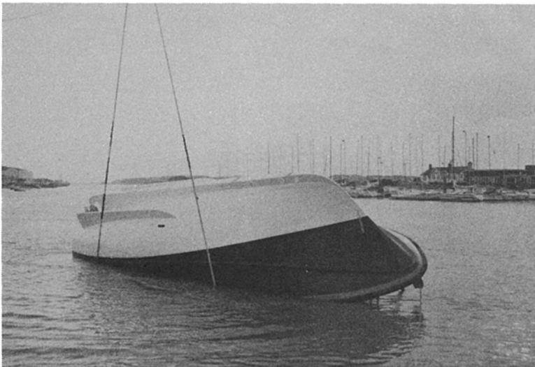
A crane tips the Lifeboat through 180°
